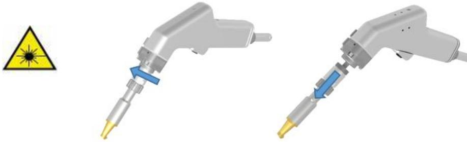
Once positioned correctly, tighten the nut and lock the nozzle tube in place, as shown in the figure. Tighten with your hand!
