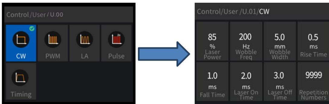
After entering the parameter selection page, single click the Confirm button to enter the parameter adjustment operation. The adjustment range of each parameter will vary. By taking the “Laser Power” change as an example for the interface adjustment, adjust the laser power from 85% to 100%. Single click the Confirm button to enter the parameter adjustment page.
