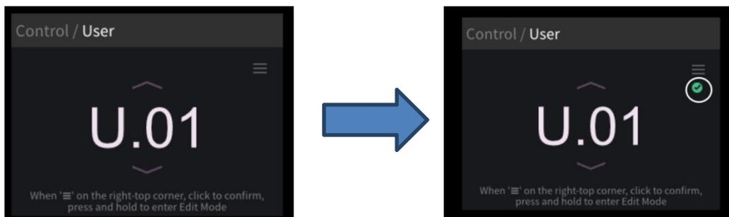
To modify the selected program number, press and hold the Confirm button on the operation panel for more than 0.5 seconds to enter the detailed parameter equipment page.
