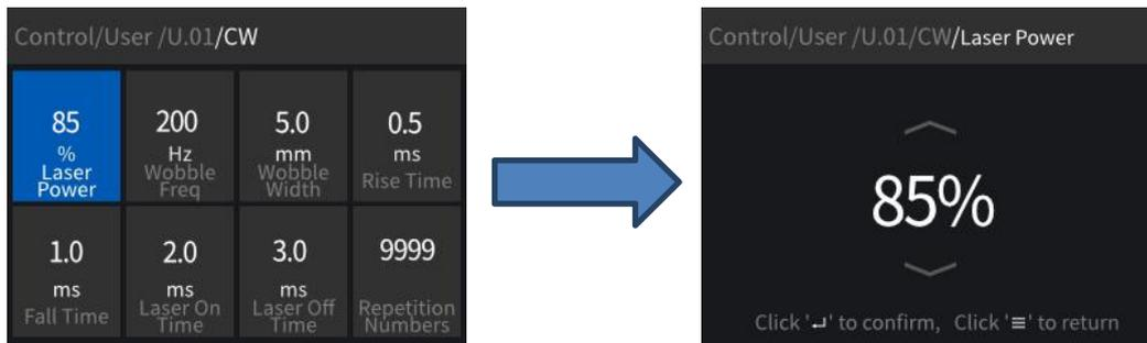
Press the up button on the operation panel to adjust the setting value to 100%. After the adjustment is completed, single click the Confirm button to save the settings.
