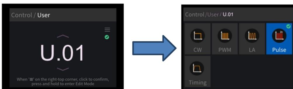
In the user program mode, you need to confirm the operating mode selected by the current program before entering the parameter setting. The system provides users with 5 operating modes to choose from.
