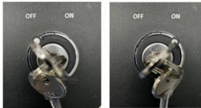
5. After the rear panel is started, the indicator and display screen will be lit. In the process of startup, the indicator light is in a color circulating state. After the completion of system starting, the indicator light will turn green in normally-on state. At this time, the equipment can enter the working state.
