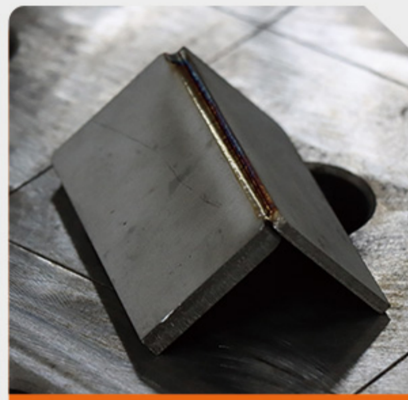
2mm-6mm SS outer corner weld
